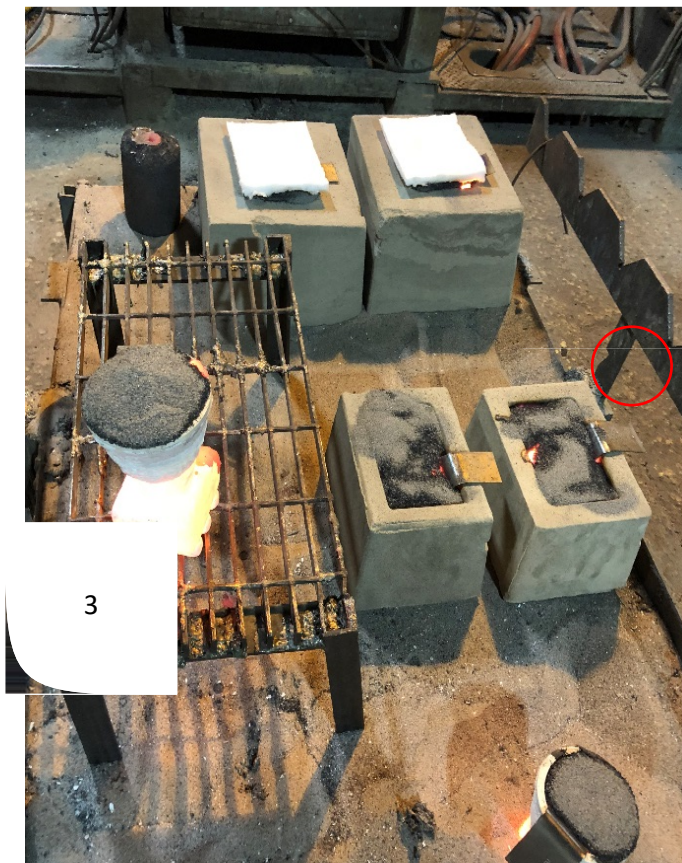
Figure 3. The experimental test bars after they were poured. All bars tagged per Table 2.
