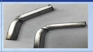
A pair of failed bend samples tested in accordance with ASTM A262, Practice E. Both the boiled and un-boiled samples failed prematurly with no ductility.
