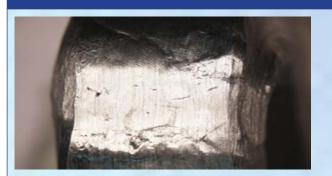
ASTM A 262, Practice E failed bend coupon. There are inclusions and fissures in the apex of the bend sample.
