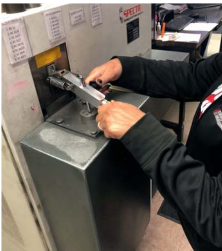
Chemical analysis being performed using an OES-DR analyzer.
