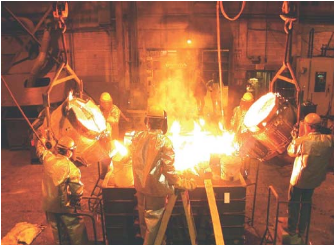
Metal being poured into air set molding sand.
