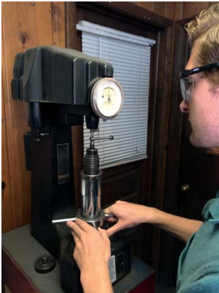
Testing a production casting for hardness with a Rockwell testing unit.
