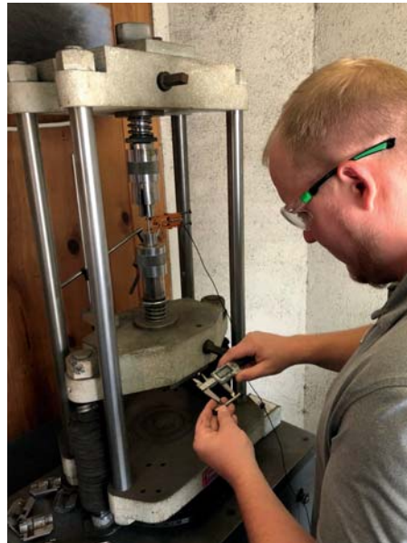
Testing of material strength via tensile testing with a universal testing machine.
