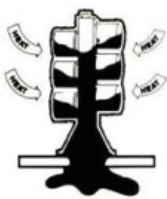
7) Melt wax out of shell mold
