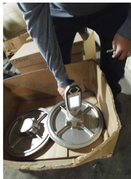
Photograph 1. PMI inspection of a cast stainless steel part verifying chemical analysis prior to shipping of product.
