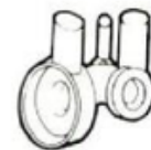
8) Remove casting from mold. Prepare for cut-off.
