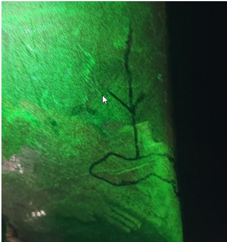
Magnetic Particle linear indication on ASTM A487, Grade CA6NM, Class A impeller
