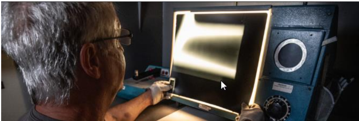
Radiograph film interpretation by a Level III Radiographer – InspecTech Corp., Milwaukee, WI
